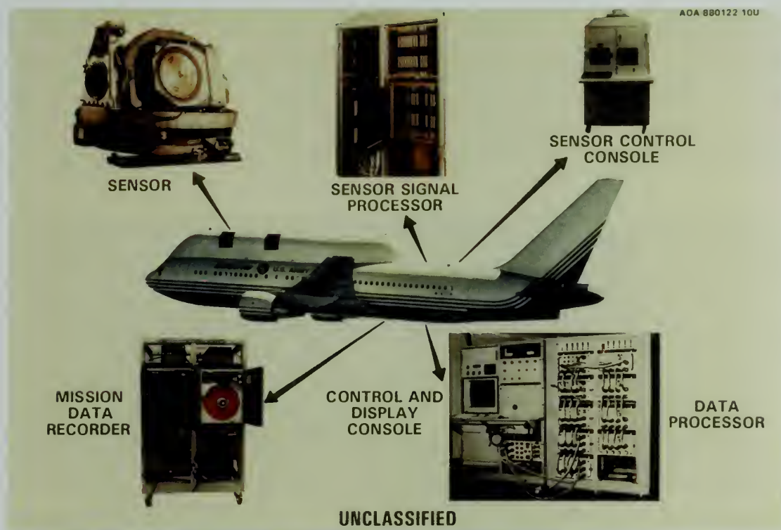
Fig. 3-25. The Airborne Surveillance Testbed, an airborne system with its heat detecting telescope, remains an important asset to Army data collection efforts. This diagram illustrates the various components of the AST system.
